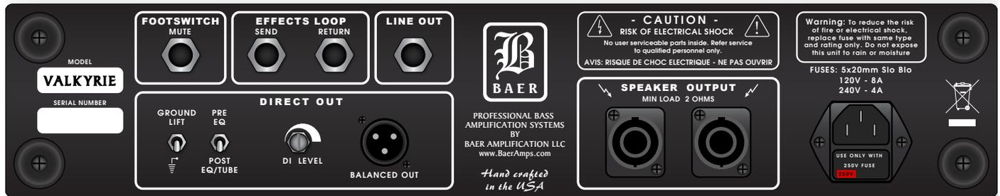
**FOOT SWITCH** - Connect the FS-1 foot switch for remote control of the MUTE function.
